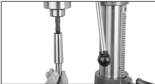
Figure 24. Inserting tooling into spindle.
